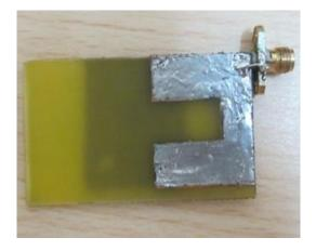
Fig.2: Body Patch Antenna showing bottom plane
