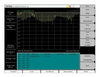
Fig.9: Measured return loss for the second antenna at 5 GHz
