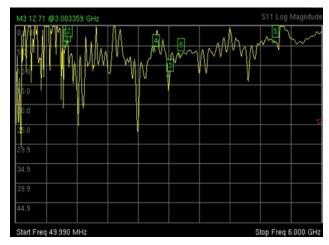
Fig.7: Measured return loss for the first antenna at 3 GHz
