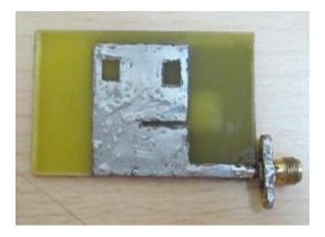
Fig.1: Body Patch Antenna showing top plane
