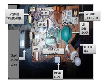
Fig.3: Hardware modules contain inbuilt ARM board, Wi-Fi and sensor values display on LCD.
