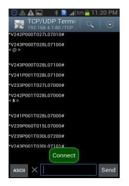
Fig.4: Android mobile to operate switching on/off device by using TCP/UDP terminal front end software it supported to Wi-Fi module.
