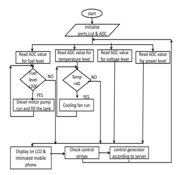
Fig.2: Following is the working flowchart that describes the overall working procedure of Industrial monitoring system in a step by step manner.
