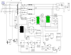
Fig.7 Simulation circuit of APF with fuzzy logic based control
