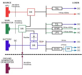
Fig.1 Structure of Aircraft Power System
