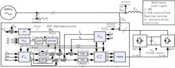
Fig.2 Structure of Active Power Filter
