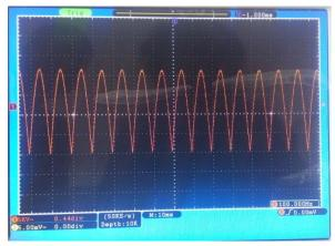
Fig.18 Digital CRO waveform of Sag voltage.
