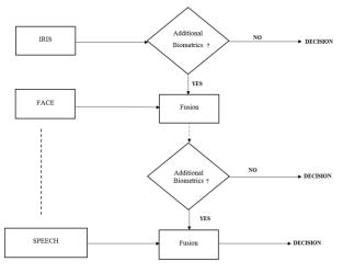
Fig.2: Serial Architecture
