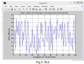
The figure shown above describes the side lobe level of the signal whose units have been described on their axis. This is the uncompensated structure with distortion. The y axis is the side lobe level and the x axis represents number of iterations.
